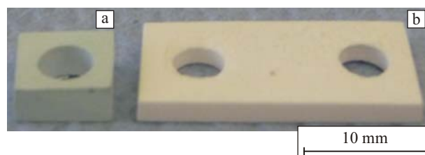
Fig. 6. Complex shape geometries of HAP (a) and \beta -TCP (b) samples after sintering.
